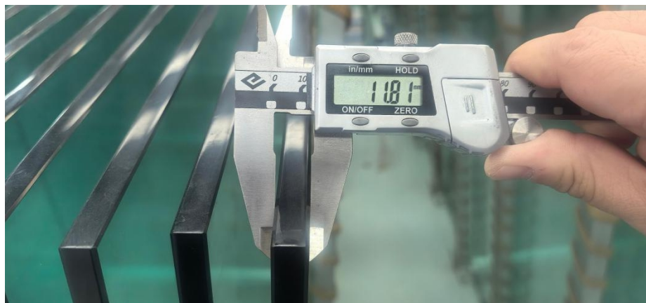
Fig.7 Measure the thickness of glass
